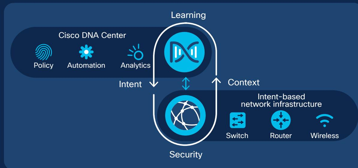
Cisco DNA is a controller-based architecture. Having Cisco DNA Center at its core, Cisco DNA provides the policy, automation, and analytics required to adapt to change, simplify and scale operations, and protect against degradation and threats. It provides 360-degree open platform extensibility to vastly increase the network's value by opening the way for new and innovative applications, processes, and solutions that are required today, and those that will be needed in the future.
