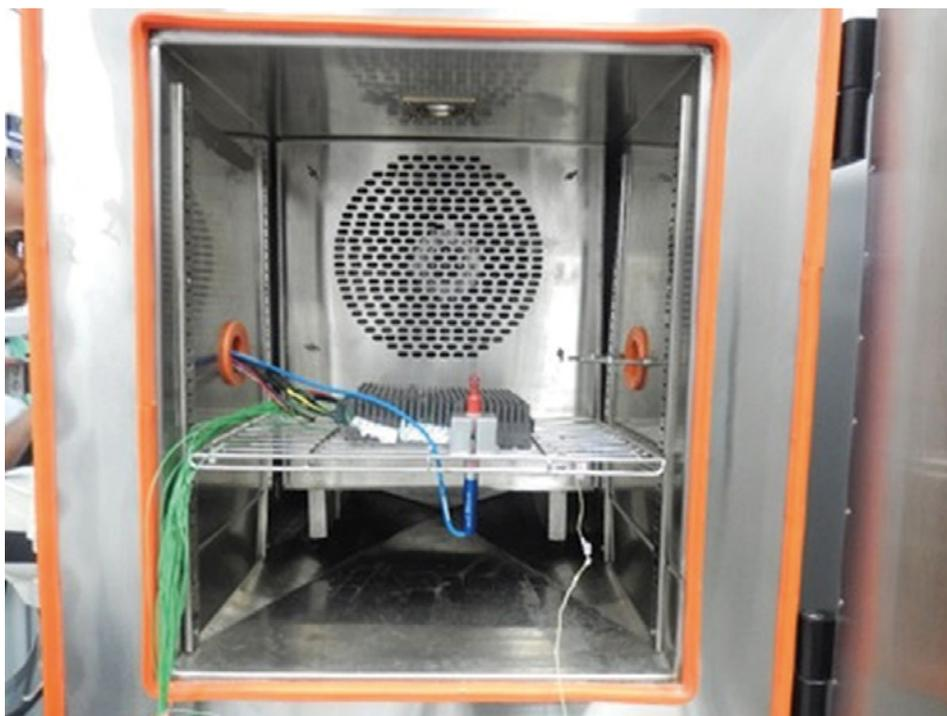
Figure 7. Thermocoupled ECU and Anemometer in the Thermal Chamber
