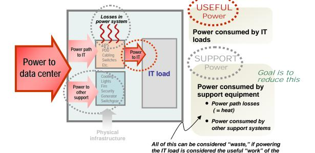
> How do high density and varying IT load reduce data center efficiency?
