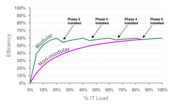
When the % IT load is well below the design value for the data center, the efficiency degrades and the data center is considered to be over-sized for that IT load. Many data centers operate in this condition – sometimes for years – typically because they are constructed for a hypothetical future IT load that has not yet been installed.
