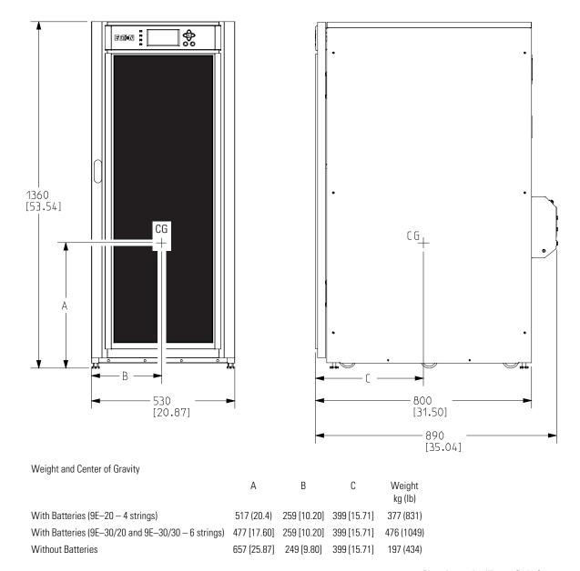
Figure 3-3. UPS Cabinet Center of Gravity
