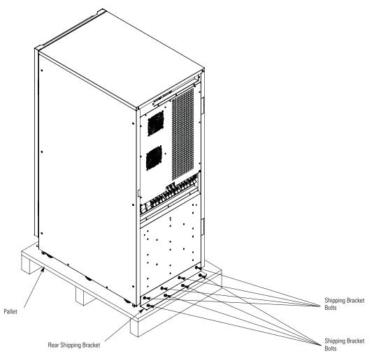
Figure 4-3. Removing the Rear Shipping Bracket
