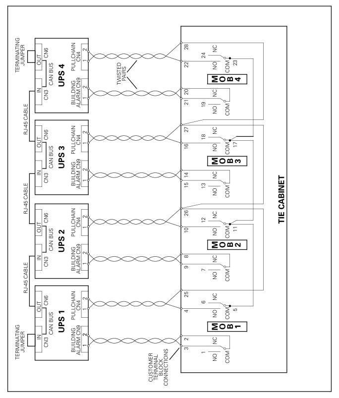
Figure 4-17. Parallel UPS Control Wiring
