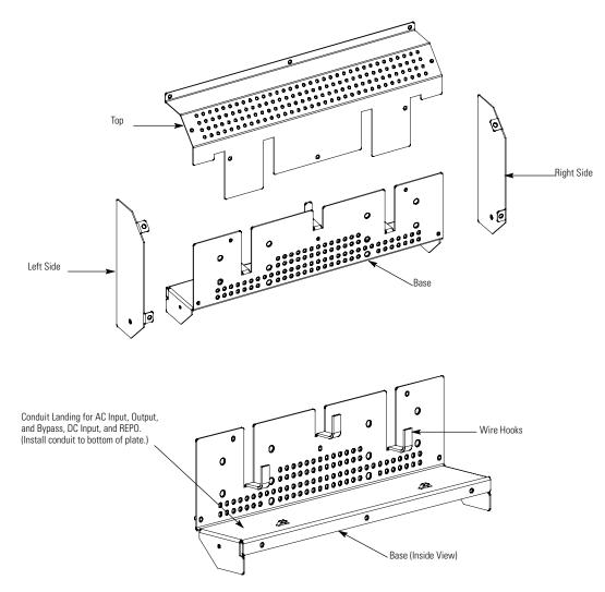
Figure 4-5. UPS Power Terminal Cover Parts
