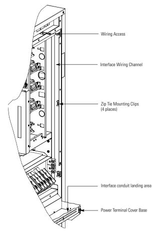
Figure 4-14. Interface Conduit Landing and Wiring Channel
