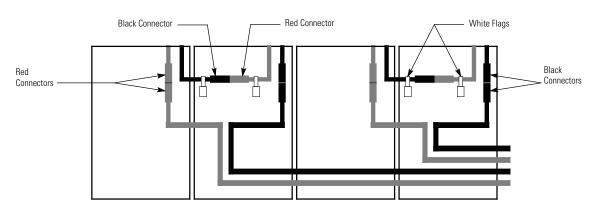
Figure 4-24. Battery String Connections
