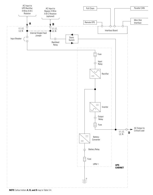
Figure 5-5. UPS System Oneline – Internal Battery
