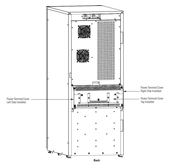
Figure 4-9. Power Terminal Cover Top Installation
