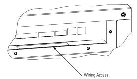
Figure 4-15. Interface Wiring Access
