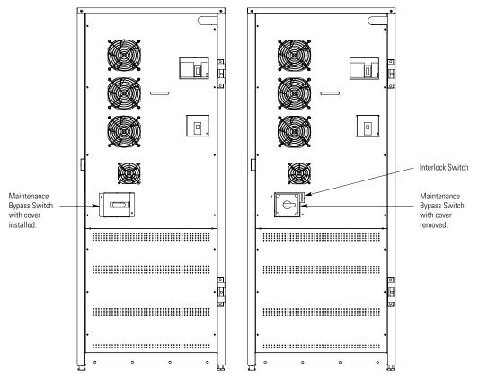
Figure 6-8. Maintenance Bypass Switch
