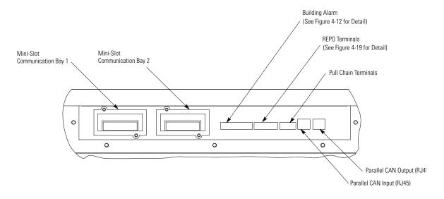
Figure 4-11. Interface Terminal Detail (Terminal Cover Removed)
