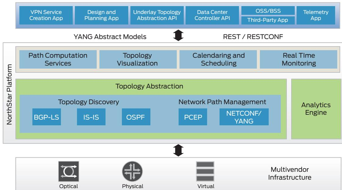
Figure 1. NorthStar architecture
